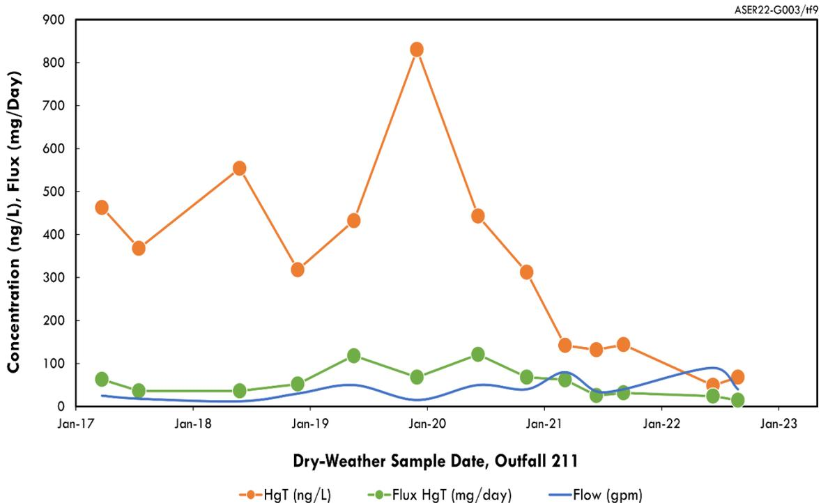
Figure 5.26. Outfall 211 dry-weather flow, concentration, and flux, 2017–2022
